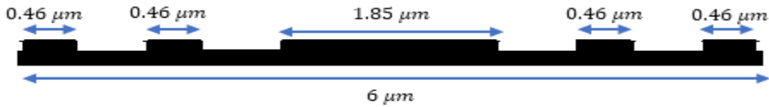
Figure11. The final binary optimized structure of the meta-lens under the numerical aperture condition (NA = 0.9).
