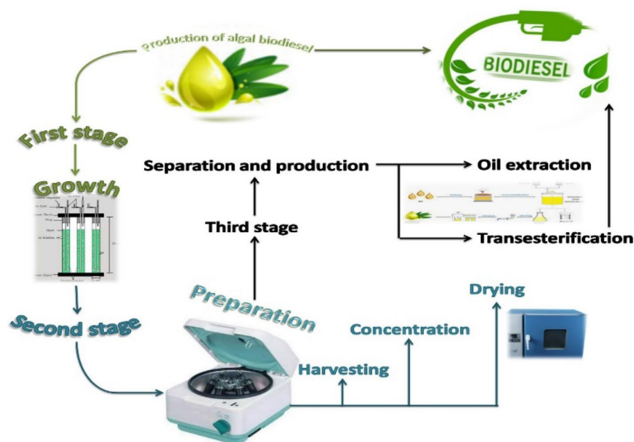
Figure 7. Stages of biodiesel production [MS Office PowerPoint 365].
