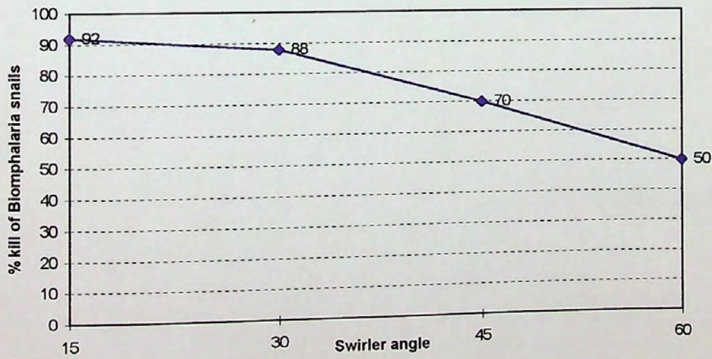
Fig. 30 : Effect of the swirling angle on the percentage kill of the Biomphalaria snails (curve)
