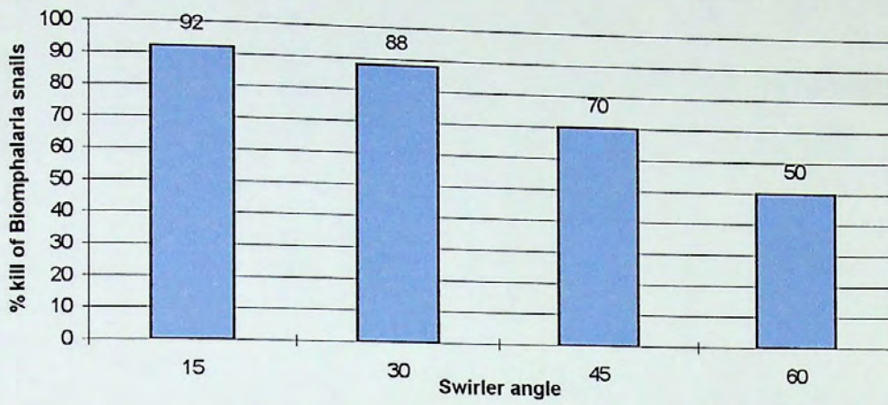
Fig. 29 : Effect of the swirling angle on the percentage kill of the Biomphalaria snails(bar chart)
