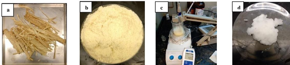
Figure 13: Isolation of Cellulose from Sugarcane Bagasse
