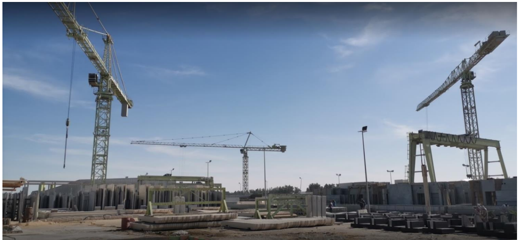
Figure 3.2: Image taken on site showing Saudi Precast Storage Yard with Fixed Cranes and Casting Bed Cranes
