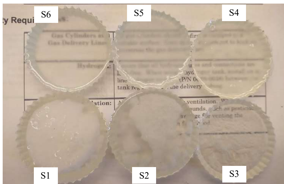
Figure 51: Transparent wood sawdust samples & wood fibers after polymer infiltration
