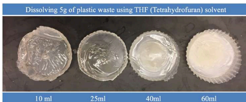
Figure 42: Plastic waste mixed in different concentrations of Tetrahydrofuran (THF)
