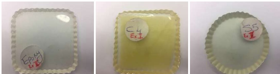
Figure 52: Epoxy sample (left), TW Casuarina using lignin modification method and epoxy (middle), & TW Sawdust using lignin modification method and epoxy (right)
