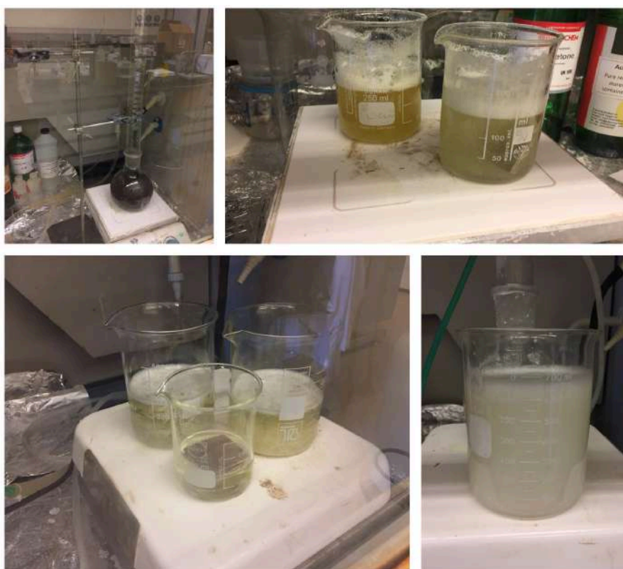
Figure 28: Chemical treatment experimental setup using flask and condenser & beakers on hot plate
