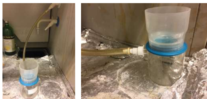
Figure 29: Dehydration setup using vacuum filter container
