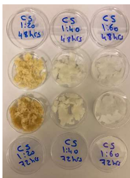
Figure 61: Color comparison for treated sawdust using commercial bleach different waste to solution ratios (1:20, 1:40, and 1:60) at 48 & 72 h of treatment
