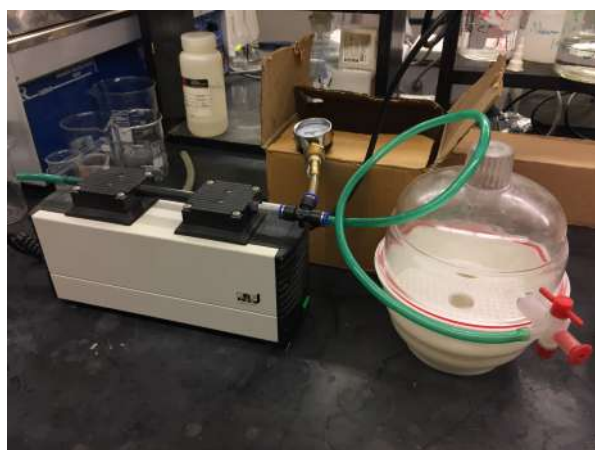
Figure 30: Vacuum infiltration setup using vacuum pump and a desiccator
