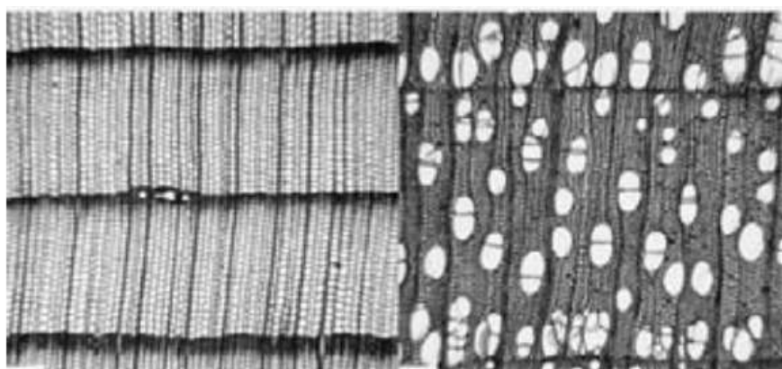
Figure 17: Cross-section of softwood (left) & hardwood (Right) showing vessel size comparison [23]
