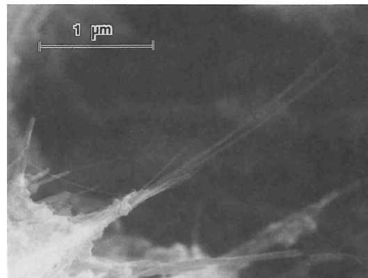
Figure 2-15 Carbon nanotubes and graphite nanoparticles grown by arc discharge.[78]
