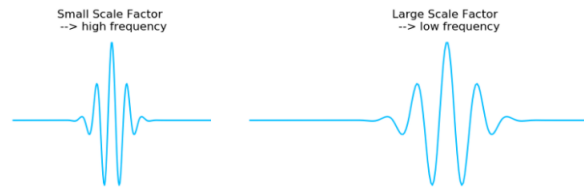
Figure 15: Demonstration of shrink and scaled Morl Wavelet, Scale is inversely proportional to frequency by Feike, S. (2020, February 10)[23]
