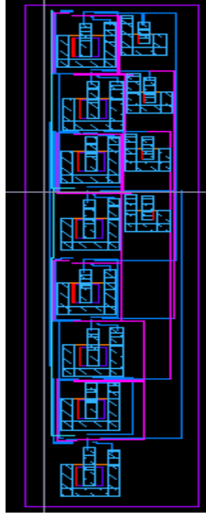
Fig.6.3 Layout of the integration switches
