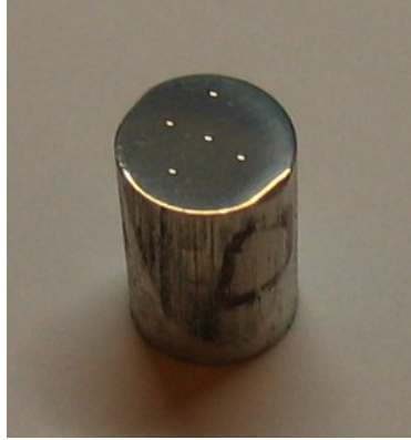
Figure 4. 8 Indentations on an extruded and polished sample
