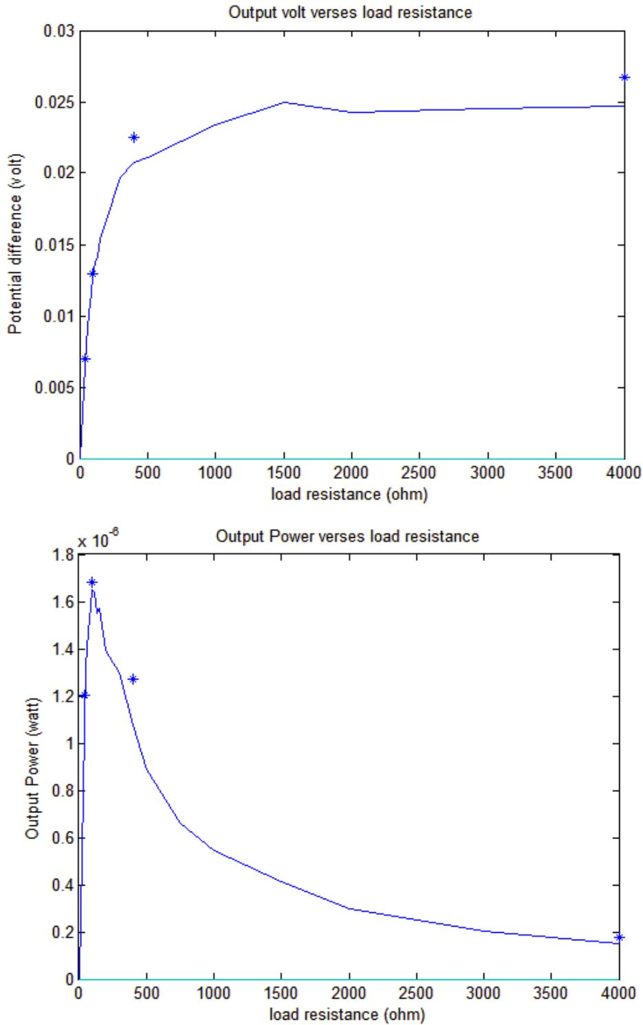
Figure 24: Graphs showing the correlation between the experimental (denoted by \*) and the model predicted values (denoted by (-)) for the volt (in the top drawing) and the power (in the bottom drawing) for different values of load resistance for wind speed of 3.2 m/s
