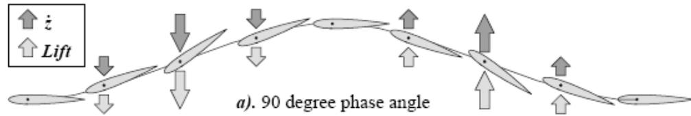
Figure 2: The lift force as it varies with the angular movement of the wing [10]
