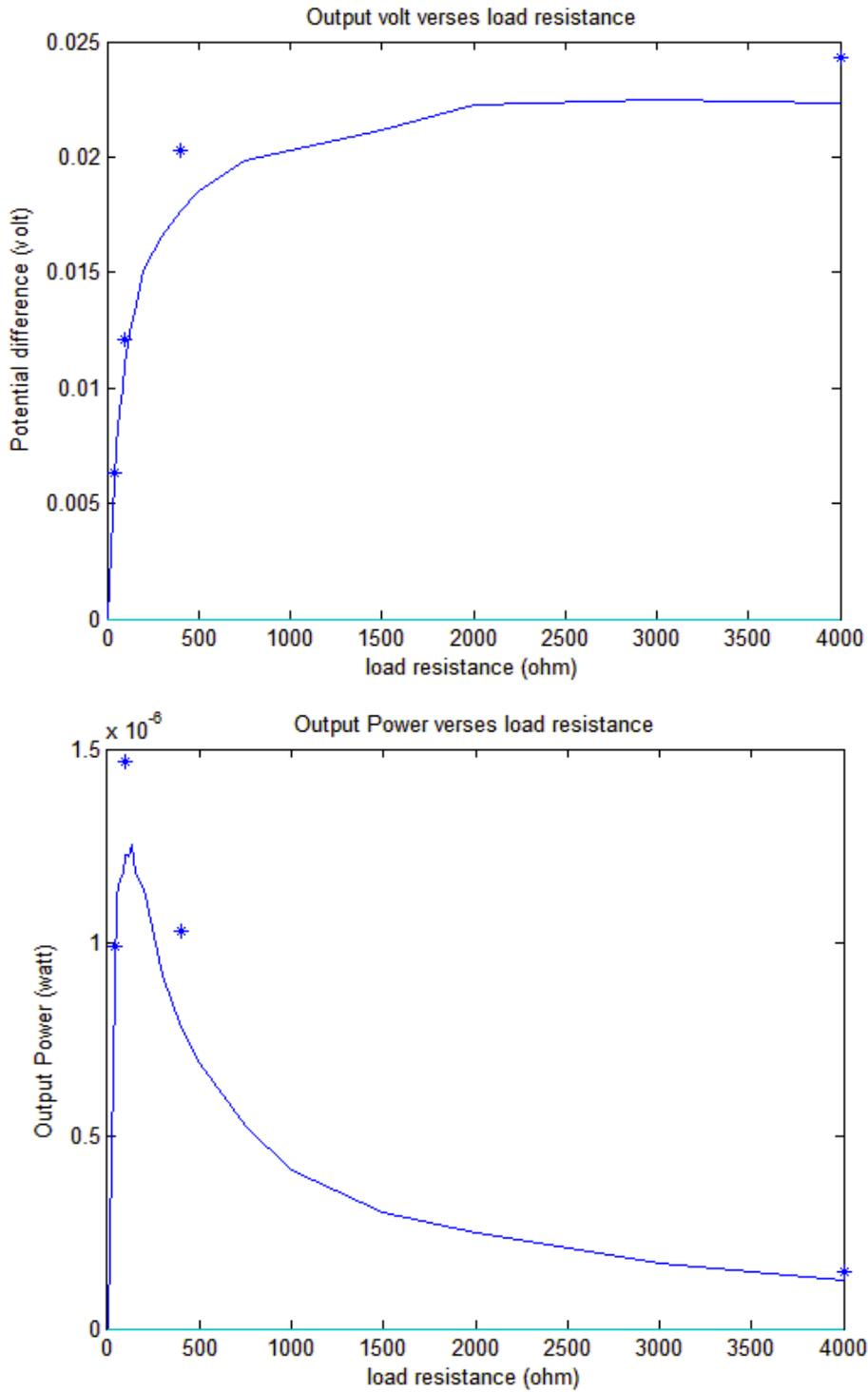
Figure 23: Graphs showing the correlation between the experimental (denoted by \*) and the model predicted values (denoted by (-)) for the volt (in the top drawing) and the power (in the bottom drawing) for different values of load resistance for wind speed of 2.7 m/s
