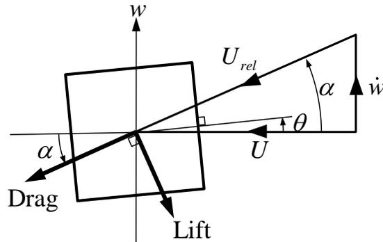
Figure 17: Air loads acting on square section
