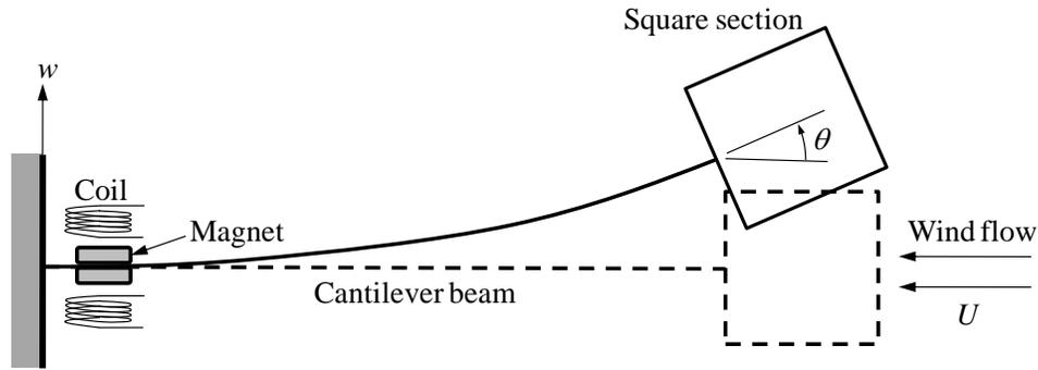
Figure 15: Schematic illustration of proposed design (top view)
