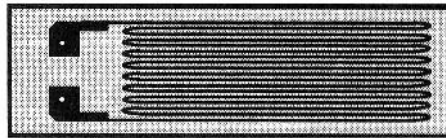
Figure 2.1: Metallic foil strain gauge (metal foil pattern –serpentine shaped- bonded on an insulating backing) [8]
