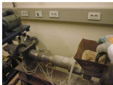
Figure 4-5: Feeding the extruder with the mixture
