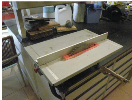
Figure 4-13: The trimmer used to cut edges
