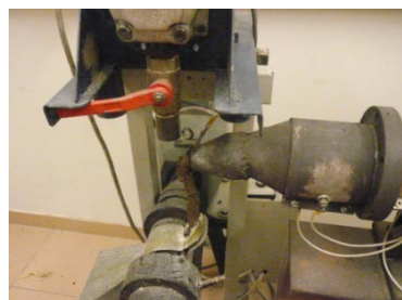
Figure 4-5: Feeding the extruder with the mixture
