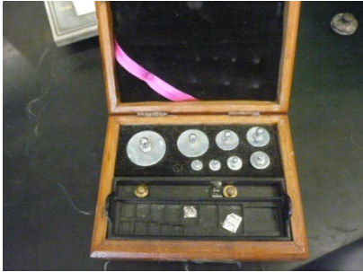
Figure 4-3: The set of standard weights used for calibration
