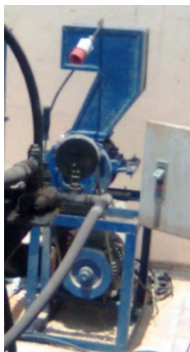
Figure 4-8: The shredder adopted in crushing the extrudates
