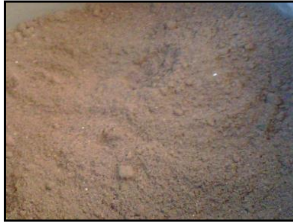
Figure 4.15: Fine particles (concrete and bricks) only
