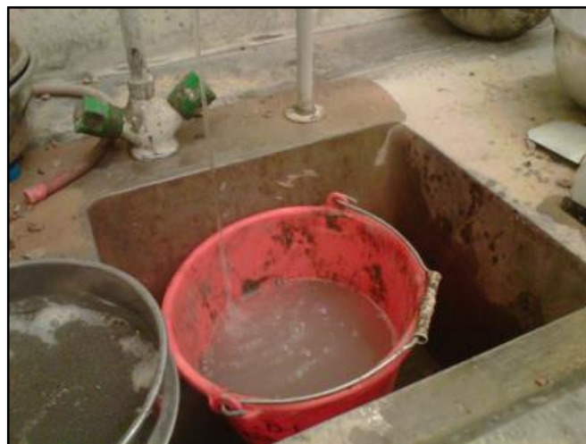
Figure 3.14: Soaking particles in water
