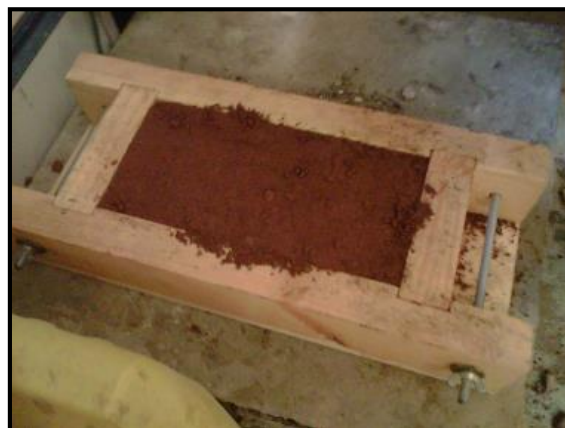
Figure 4.17: Red bricks in molds
