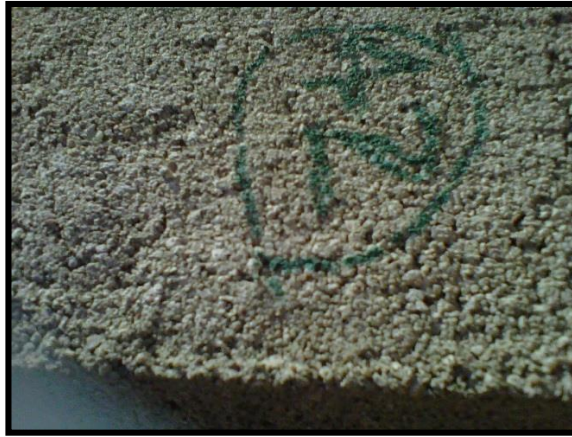
Figure 4.9: Lack of Fine particles/high porosity
