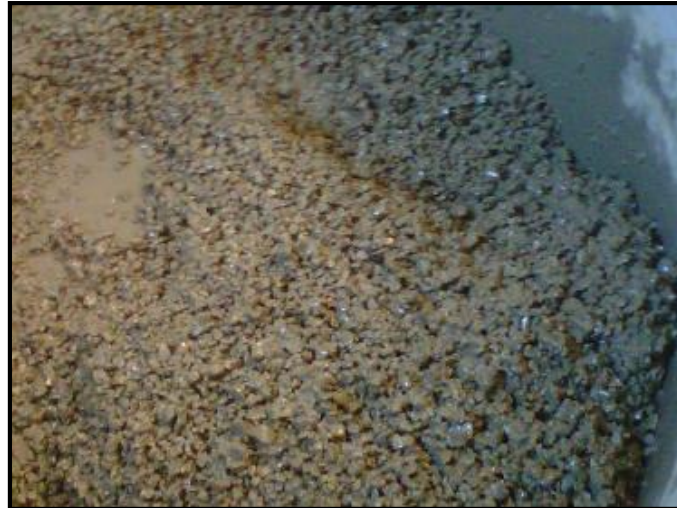
Figure 4.13: Large particles with no gradation
