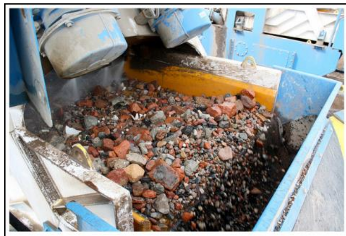
Figure 3.12: Washing recycled aggregates (Craven, 2009)
