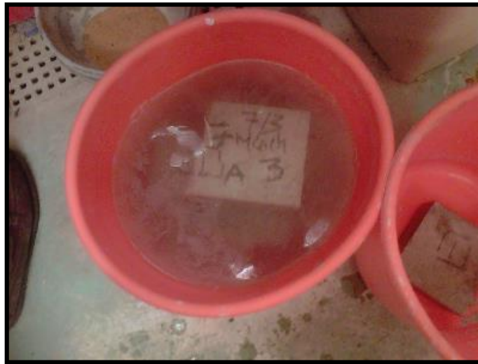
Figure 3.27: specimen curing in water
