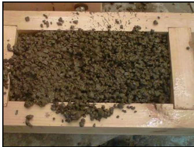
Figure 4.14: Placing the large particle sizes in the molds
