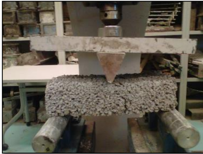
Figure 3.26: Flexural strength machine used
