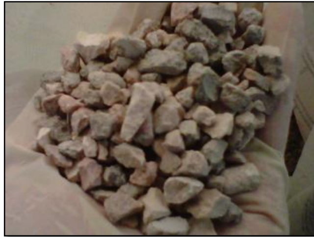
Figure 3.17: particles passing sieve (No. 1) and retained on sieve (No. \frac{3}{4} )
