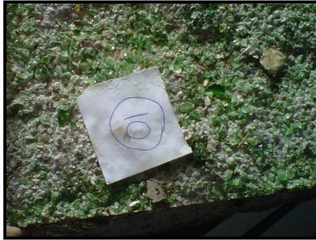
Figure 4.5: waste glass used in the mix
