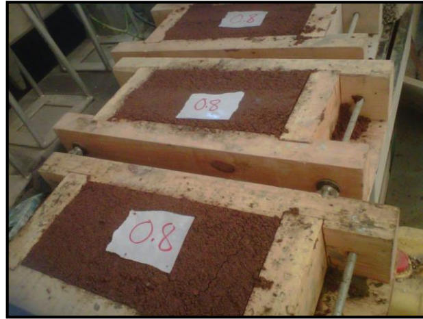
Figure 4.18: Red bricks with w/c = 0.8
