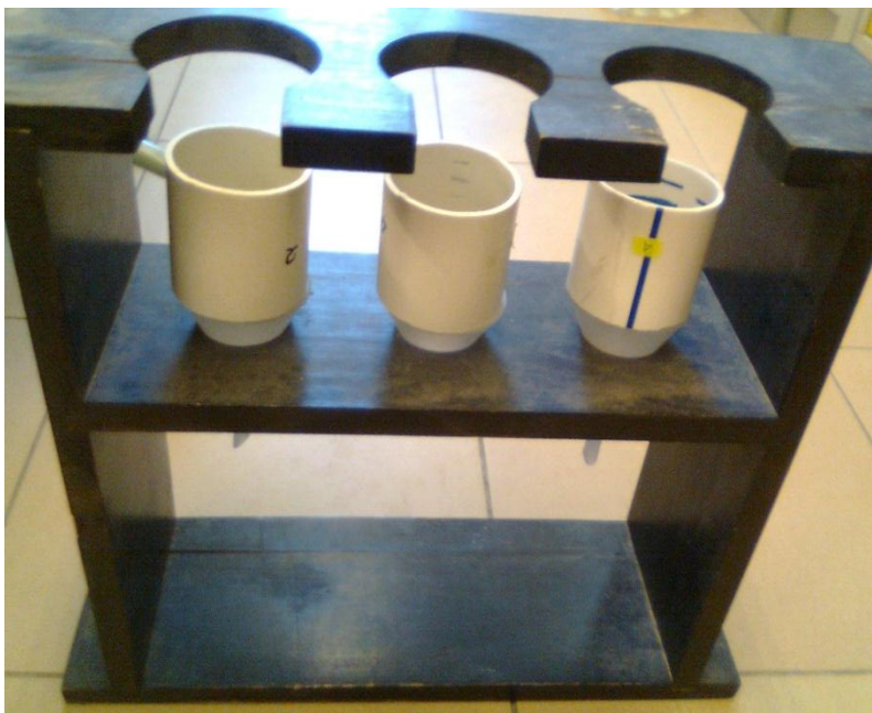
Figure 3-1 – Soil Columns Used in Bacteria Growth and Survival Experiments
