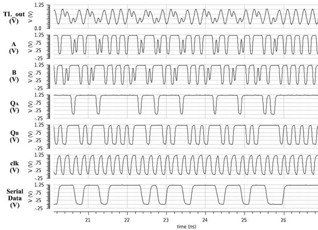
Figure 4.32 The post layout simulated waveforms of the signals in the decoder circuit (see Figure 4.12)
