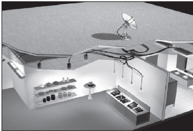
Figure 3. 5 – Conceptual Illustration of the Hybrid Solar Lighting – “Hybrid Solar Lighting Illuminates Energy Savings for Government Facilities”, n.d
