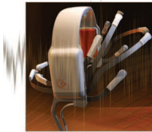
Figure 3.6: Emotiv headset with 16 electrodes to cover the different parts of the brain.
