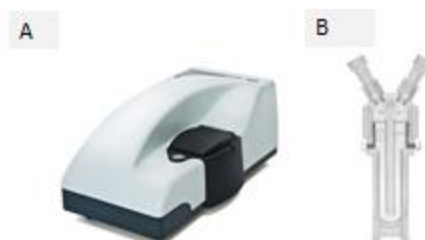
Fig2.14. (a) Zeta sizer and zeta potential Malvern apparatus (b) potential cuvette [108][109]
