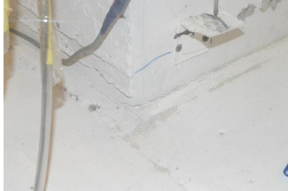
Figure 5.99: starting slipping from base of column at 1.3\Delta y
