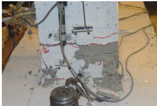
Figure 5.68: CSF-0-7.5-NCrushing concrete cover at (2.197 \Delta y )
