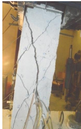
Figure 5.100: Specimen CSS-15-E at the tension direction of 2.2\Delta y
