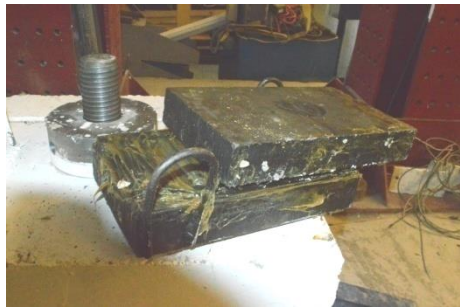
Figure 4.19: High strength upper steel plate with lubricate
