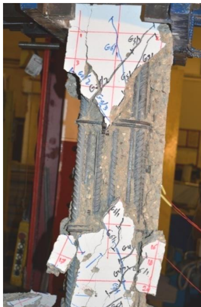
Figure 5.137: CSS 40-ECrushing column concrete cover ( 4.8\Delta y )
