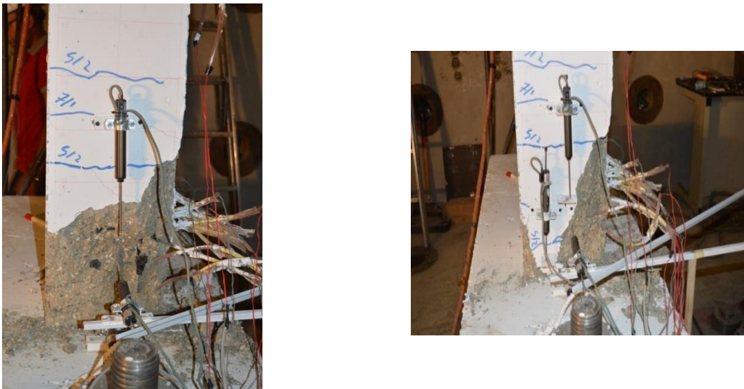
Figure 5.18: CSF-10-16-N Compression and tension of loading of 3.72\Delta y
