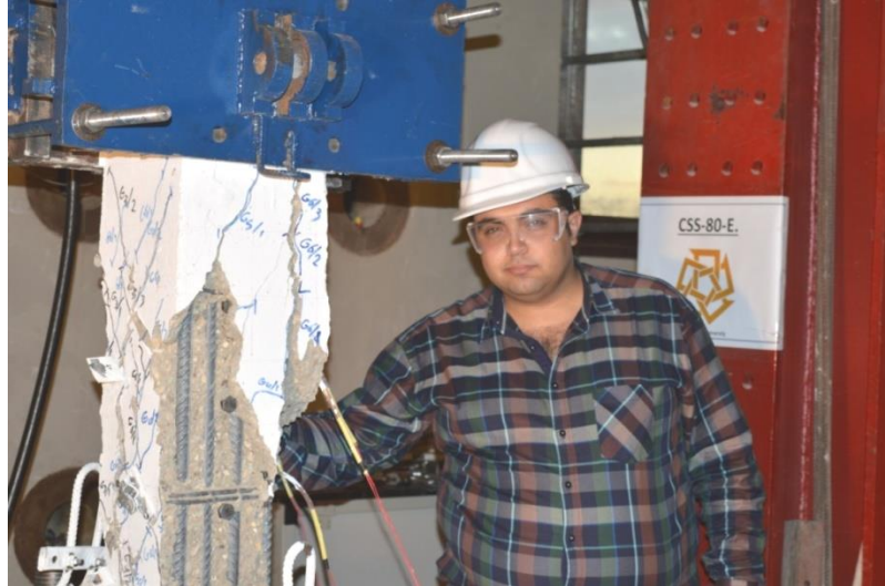
Figure 5.170: CSS-80-E failure end of the test
