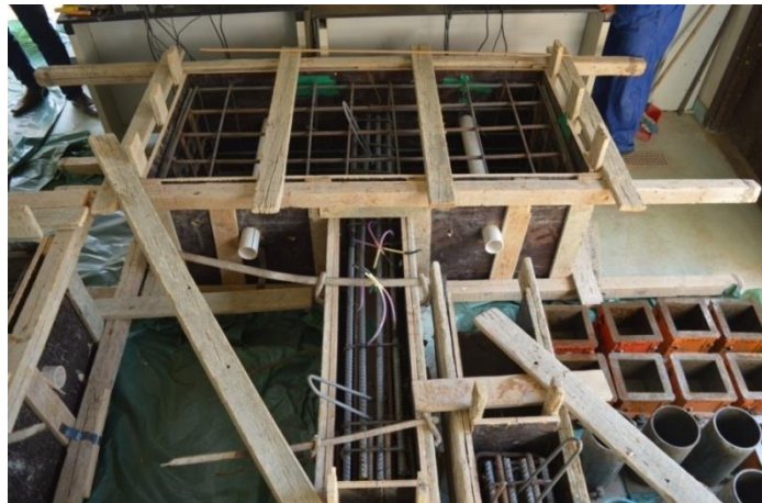
Figure 4.23: Fixing the specimen frame
