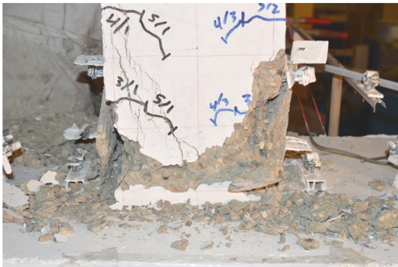
Figure 5.222: CSF-80-E Crushing concrete cover (2.85 \Delta y )
