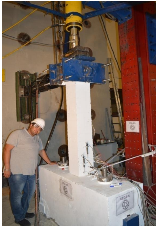
Figure 4.9: Modern building test specimen arrangement of LVDT
