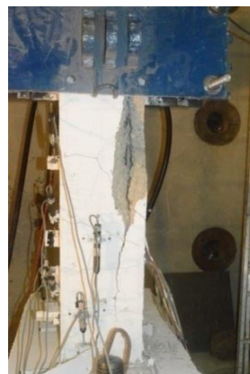
Figure 5.101: CSS-15-E Crushing concrete cover at the compression side at displacement of 2.85\Delta y
