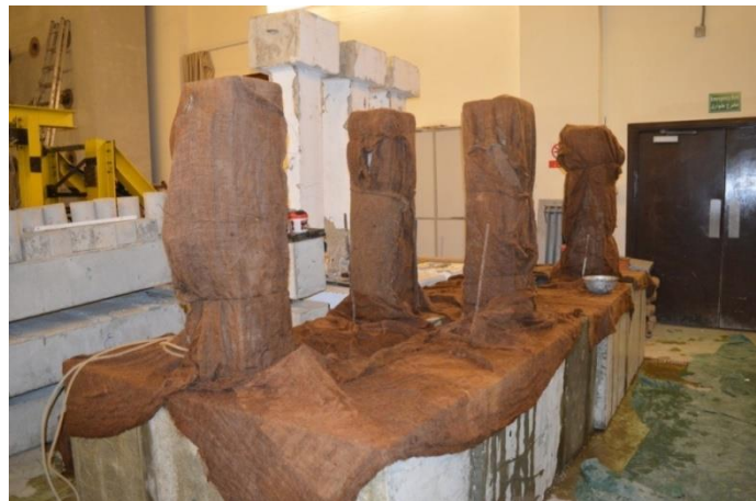
Figure 4.35: Curing stage of specimens and their sample cylinder and cub samples
