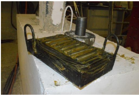
Figure 4.18: High strength steel rods with lubricate
