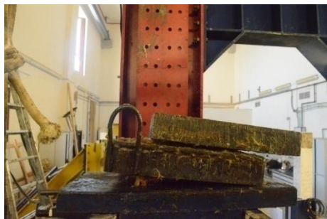
Figure 4.19: High strength upper steel plate with lubricate
