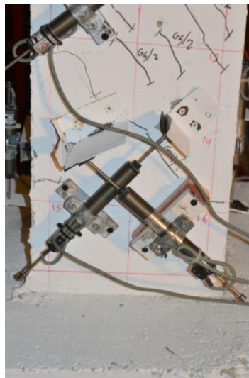
Figure 5.114: CSS-20-E Start slipping at 2.2\Delta y
