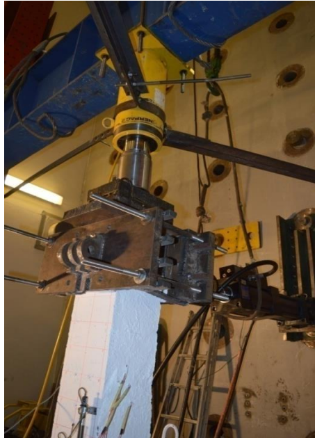
Figure 4.16: Column head fixation setup
