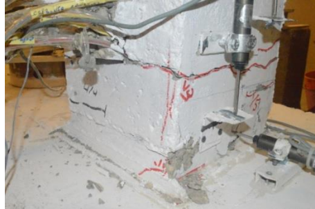
Figure 5.67: CSF-0-7.5-NCrack opening width 3mm at 2.197 \Delta y
