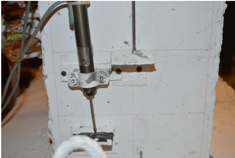
Figure 5.11: Specimen CSF-10-16-N at initial displacement (Hair cracking)
