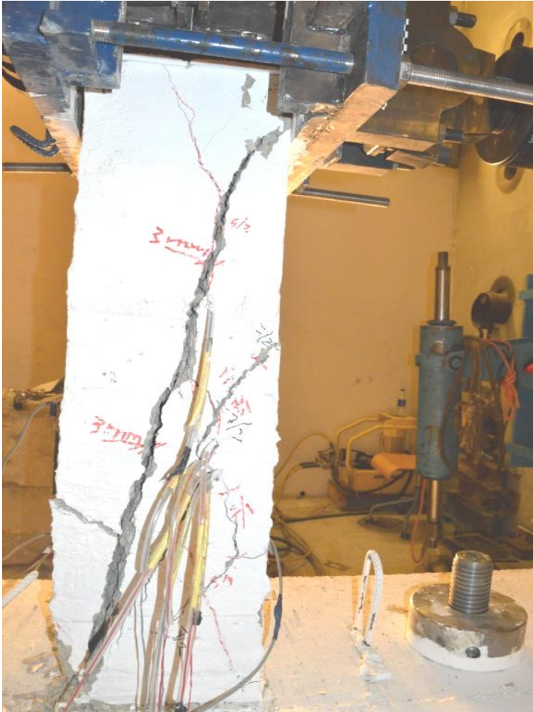
Figure 5.153: CSS-60-E failure at the end of the test
