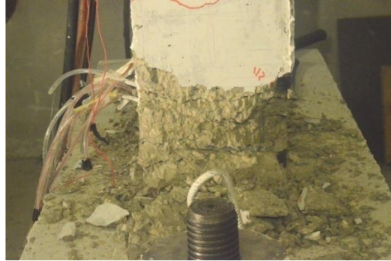
Figure 5.45: CSF-10-75 Compression side at (2.85\Delta y)
