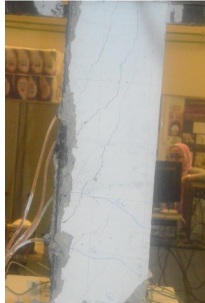
Figure 5.103: CSS-15-E Compression and tension of loading of 3.72\Delta y
