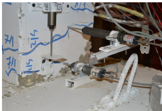
Figure 5.16: CSF-10-16-NCrushing concrete cover at 2.85\Delta y
