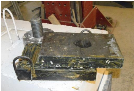
Figure 4.19: High strength upper steel plate with lubricate
