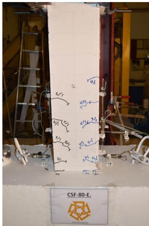
Figure 5.219: CSF-80-E Start slipping at \Delta y
