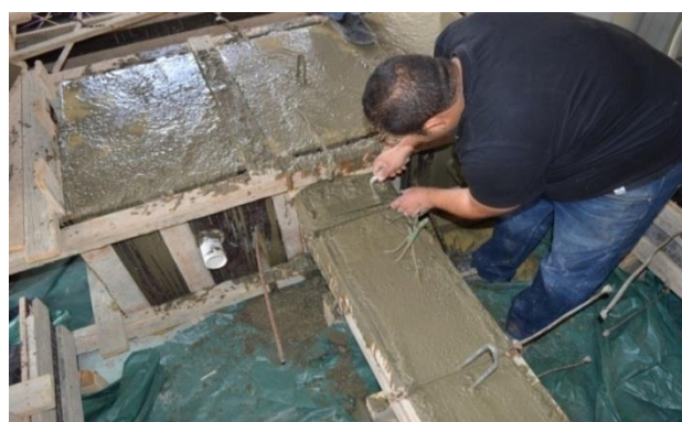
Figure4.31: Ensuring the strain gages places
