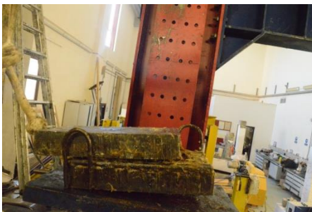
Figure 4.19: High strength upper steel plate with lubricate
