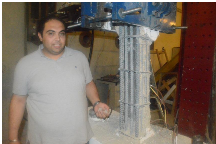
Figure 5.9: Damage pattern of specimen CSS15-E-25
