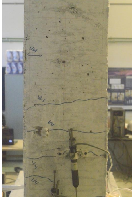
Figure 5.39: CSF-10-75 Tension side at \Delta y
