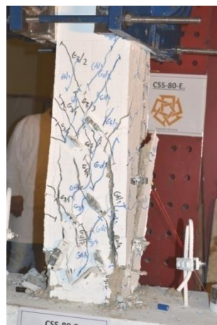
Figure 5.169: CSS-80-ECrushing column concrete cover at (2.85 \Delta y )
