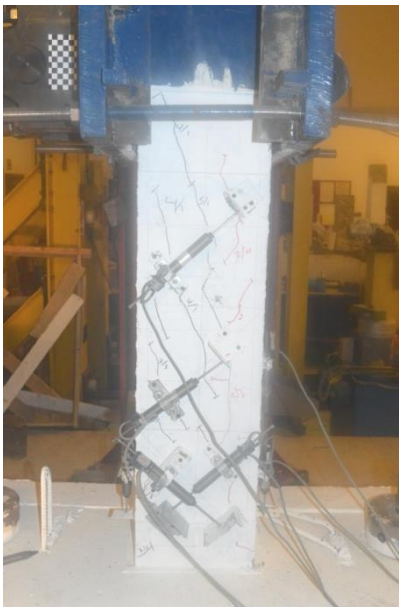
Figure 5.149: CSS 60E Start slipping at 2.2\Delta y
