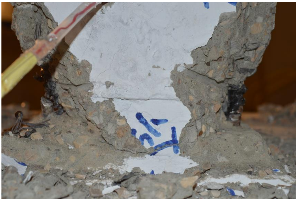
Figure 5.202: Classical tension failure 4.8\Delta y
