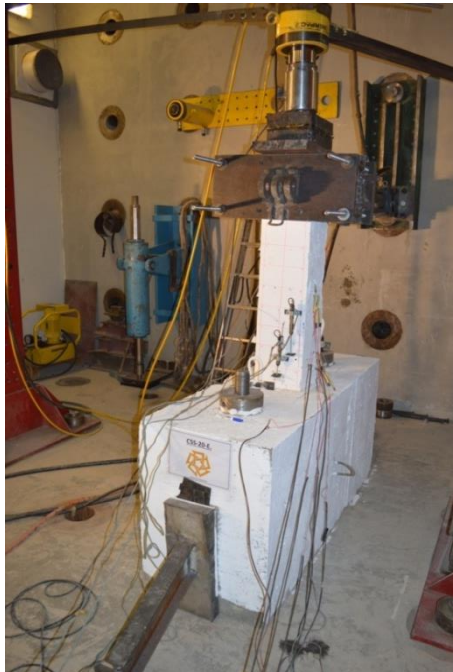
Figure 4.16: Column head fixation setup
