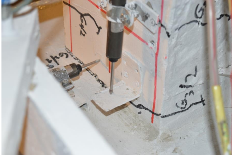
Figure 5.198: CSF-15-E starting slipping from base of column at 0.5\Delta y
