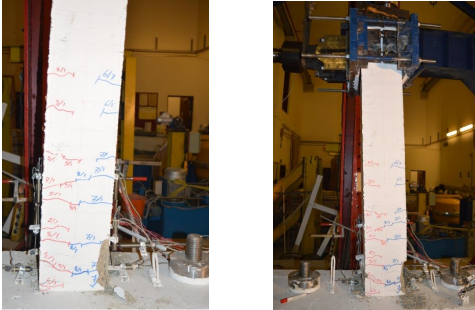
Figure 5.18: CSF-10-16-N Compression and tension of loading of 3.72\Delta y
