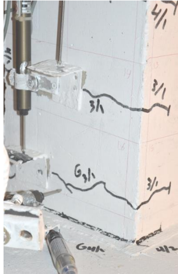
Figure 5.219: CSF-80-E Start slipping at \Delta y
