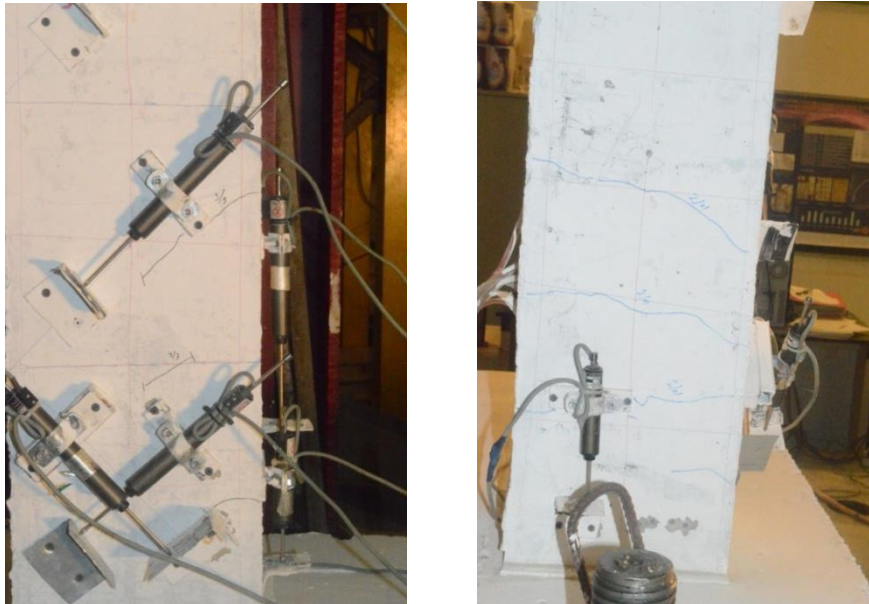
Figure 5.98: Specimen CSS-15-E at initial displacement (hair cracking)
