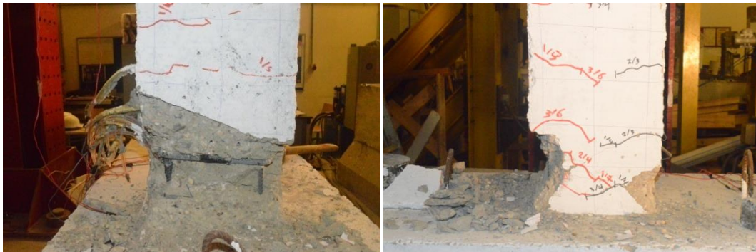
Figure 5.68: CSF-0-7.5-NCrushing concrete cover at (2.197 \Delta y )
