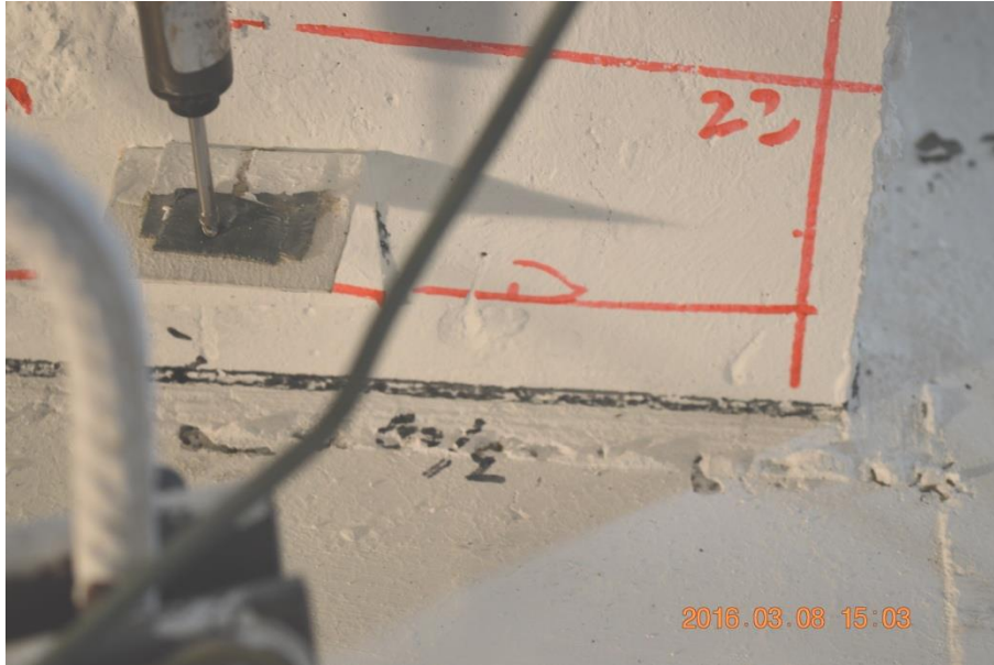
Figure 5.132: CSS 40-E start slipping at \Delta y
