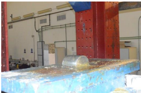
Figure 4.20: Head mechanism of load transfer
