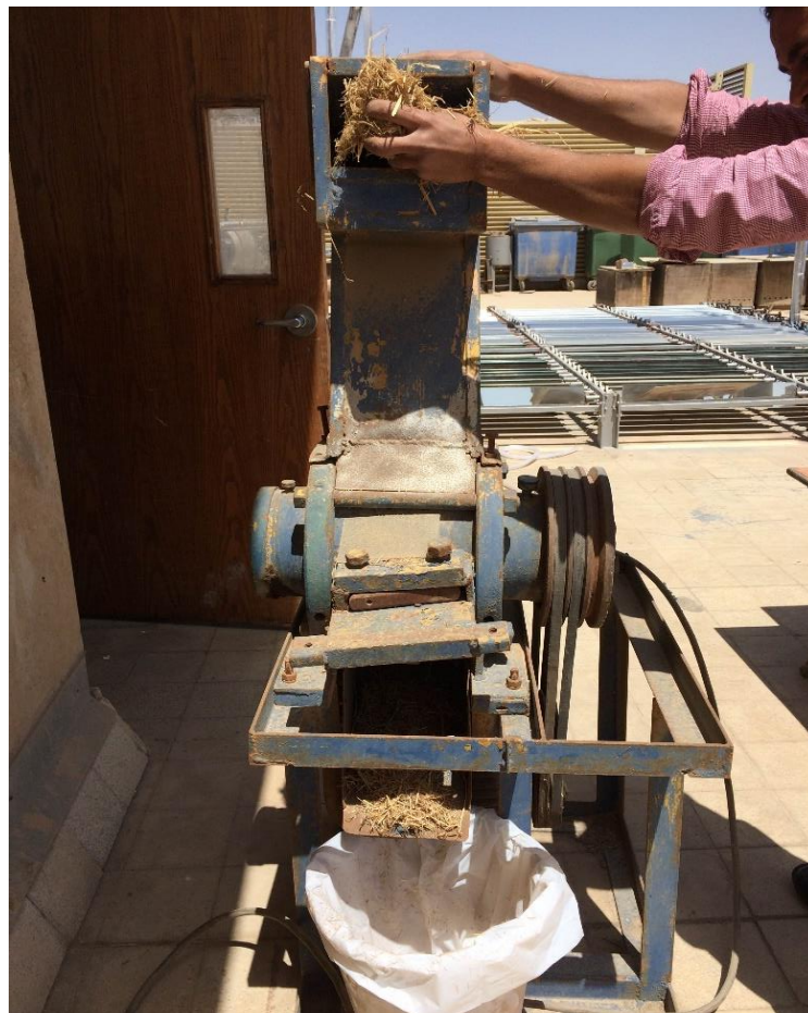
Figure 4 - Feeding large rice straws into the cutting machine to be cut into smaller straws
