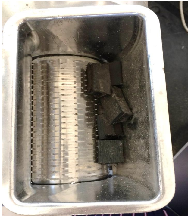
Figure 9 - Cutting tires into finer grains using cheese machine
