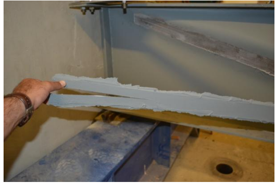
Figure 15: De-lamination of CFRP strips (SG-3.5-135-2)
