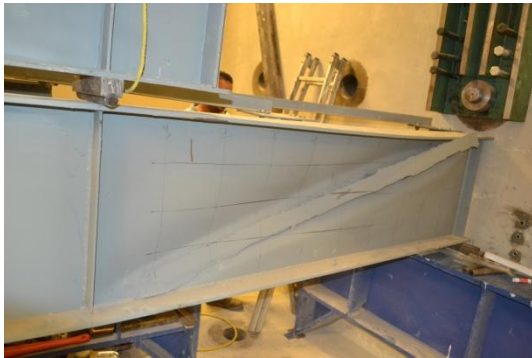
Figure 14: Web buckling and de-bonding of CFRP (SG-3.5-135-2)
