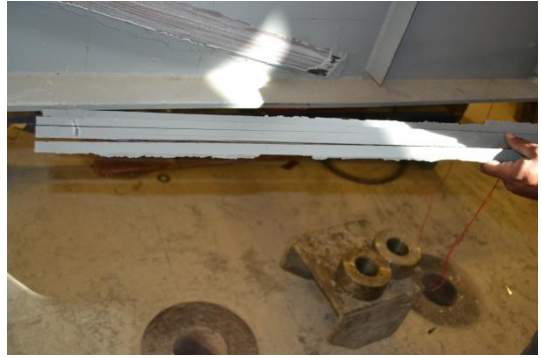
Figure 13: De-lamination in detached CFRP (SG-3.5-135-1)
