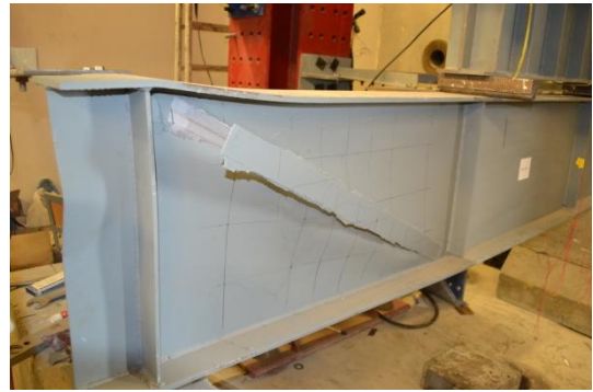
Figure 9: Web buckling and de-bonding of CFRP (SG-2-135-1)
