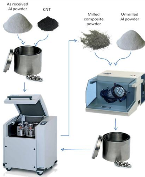
Figure 1: Experimental Procedure for preparing single and dual matrix Al-CNT powders
