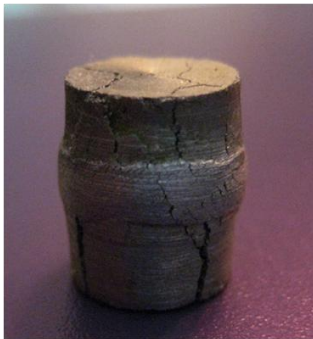
Figure 5: Failure of a 5-layer sample
