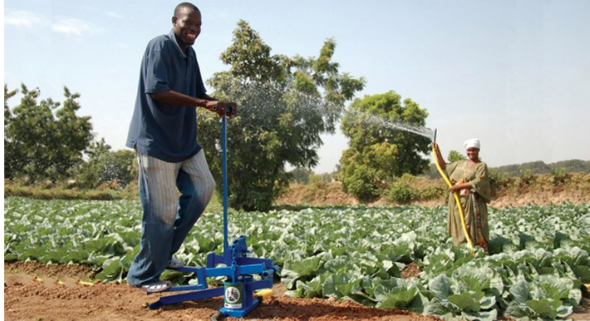
Figure 4.16 Operation of a Treadle pump
