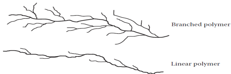
Figure 6: Schematic representation of branched and linear polymers showing the larger volume swept out by the branched structure, resulting in its lower density. Branches of the main backbone are indicated by narrower lines; they have no direct proportional relationship to cross-sectional dimensions. (From Brown, W.E., Plastics in Food Packaging: Properties, Design and Fabrication , Marcel Dekker, New York, p. 106, 1992)
