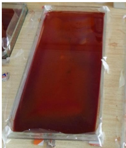
Figure 30: The corona treated LDPE films were spread on the interior surface of glass molds (dimensions, 37x19.4 cm) with different concentrations of GSE or GSKE solutions.
