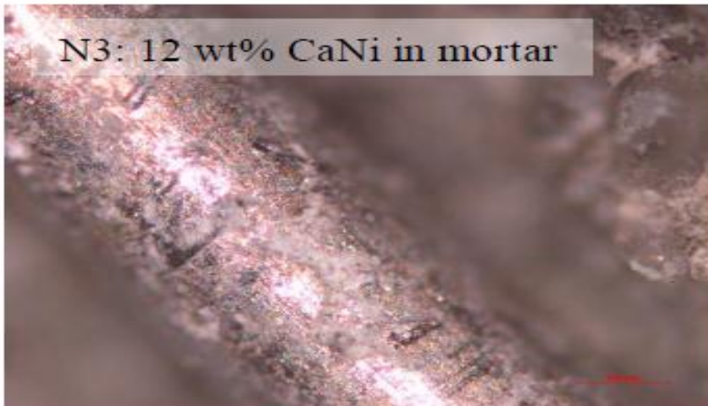
Figure 2-11 Reflective microscope image showing steel wire condition in mortar after corrosion test for capsule containing sample (Reinke 2012)
