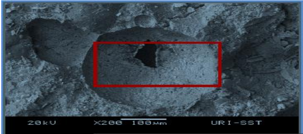
Figure 2-14 SEM images of a broken capsule after crack passes through it (Reinke 2012)
