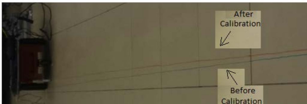
Figure 58: The robot path before correction (green) and after correction (red).
