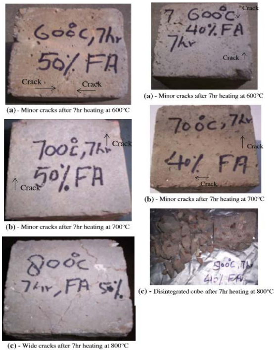
Figure 2.8 showing different patterns of cracking upon failure due to different heating scenarios (Khan et al. 2011)
