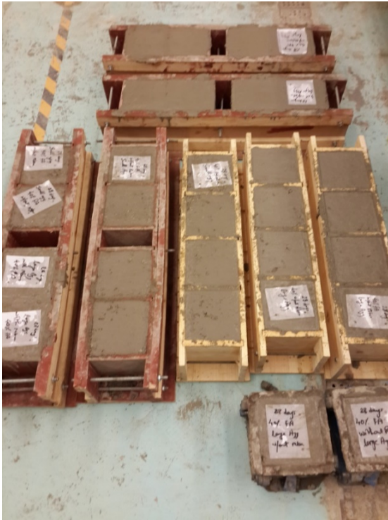
Figure 3.8: A photo of samples left for 24 hours after pouring before removing from moulds
