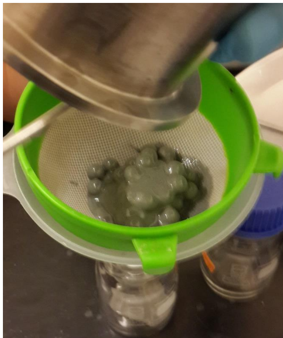
Figure 35 Transferring the paste from the milling container to the glass jar
