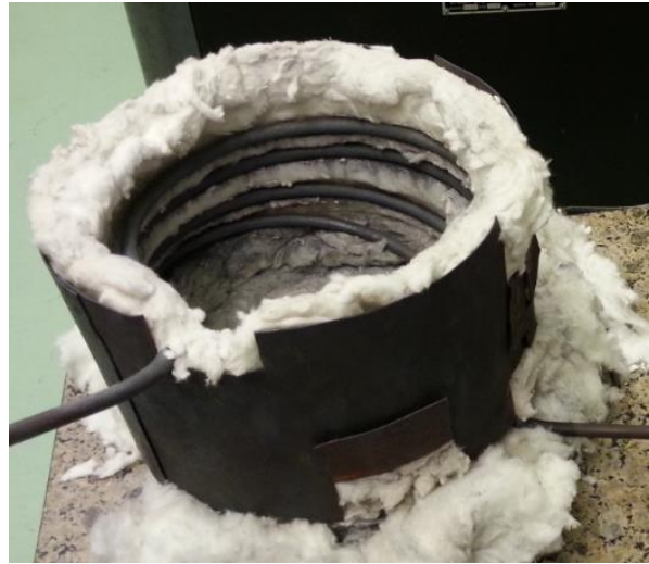
Figure 20 Electric Heating Coil - Sintering Step
