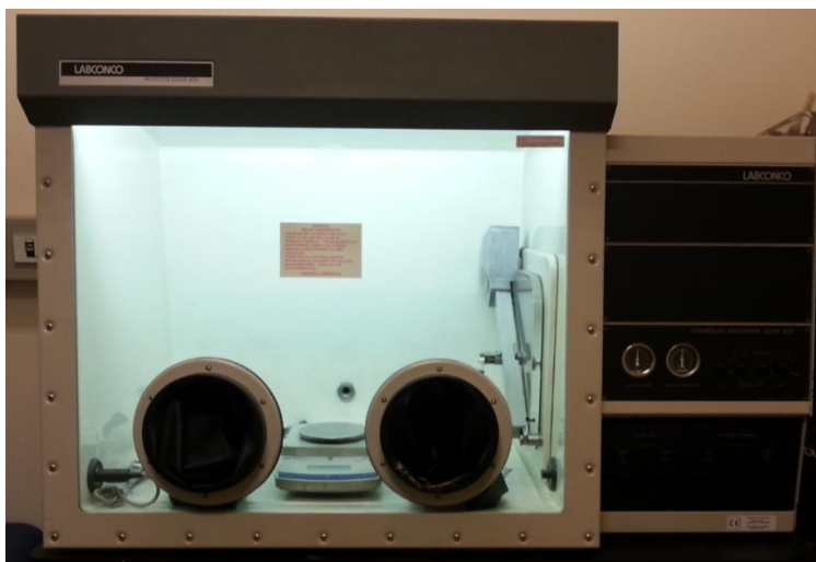
Figure 13 Glovebox: Exterior View
