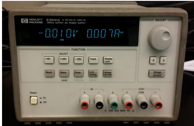
Figure 27 DC Generator used in Electrical Resistivity Measurement
