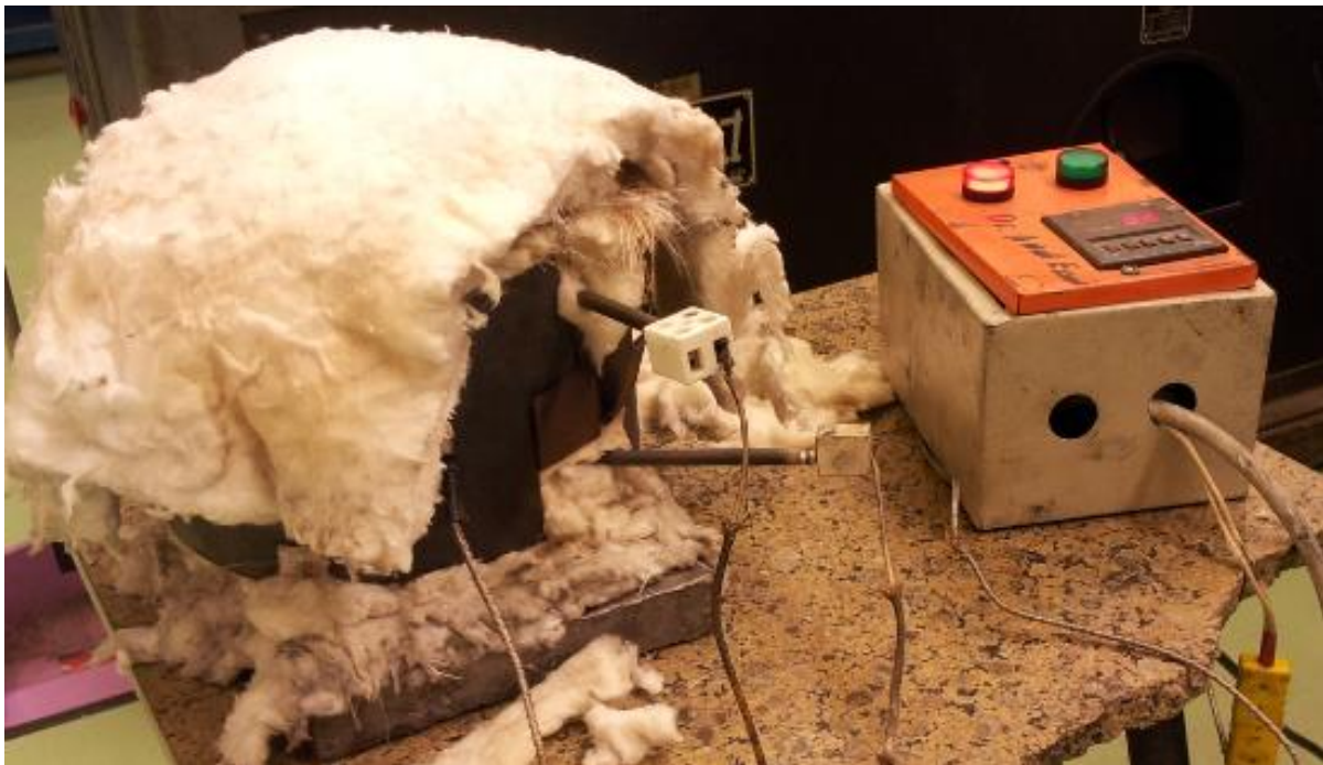
Figure 21 Sintering Step: Left: the electric coil with the die inside and covered by white insulator. Right: Electric Heater Controller
