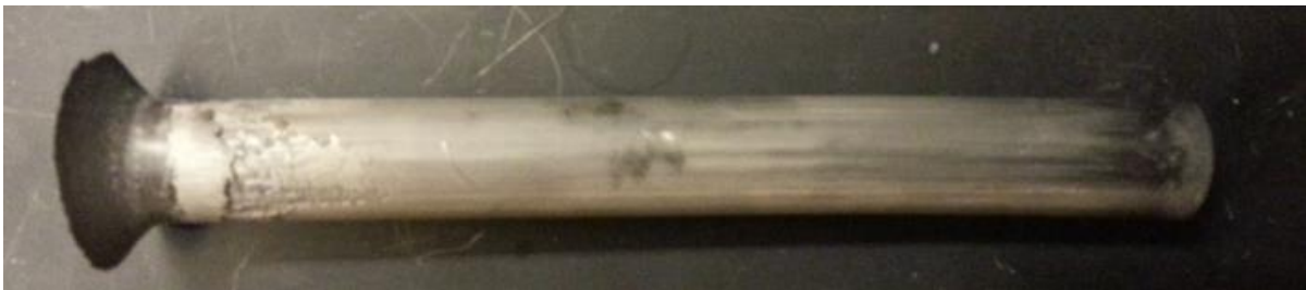
Figure 23 Extrudate sample after being removed from the die.
