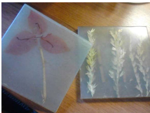
Figure 3.6: Samples of two Styrofoam-based Panels Pressed with Plants in between.
