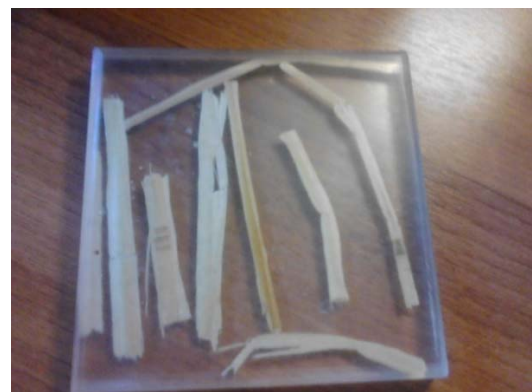
Figure 3.7: Sample with Acrylic Sheets with Wooden Straws in between
