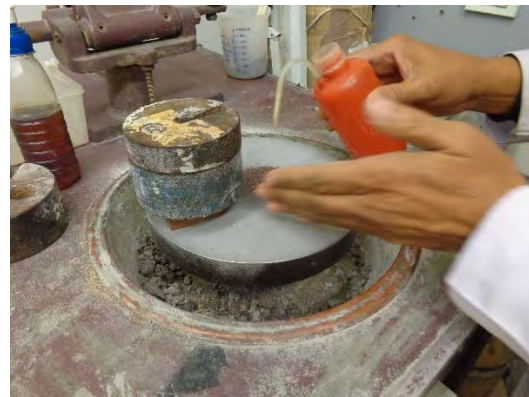
Figure 4.16: Lab Assistant Placing Sample on Rotating Disk
