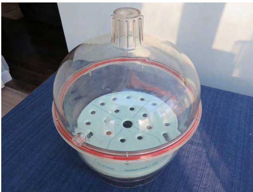
Figure 3.28: Humidity Chamber, for Water Absorption Test
