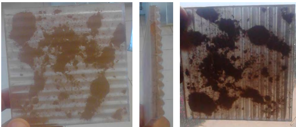
Figure 3.8: Sample of Two Acrylic Sheets Pressed with Redbrick Powder in between. One Side Smooth & the Other Zig-Zag Formed.
