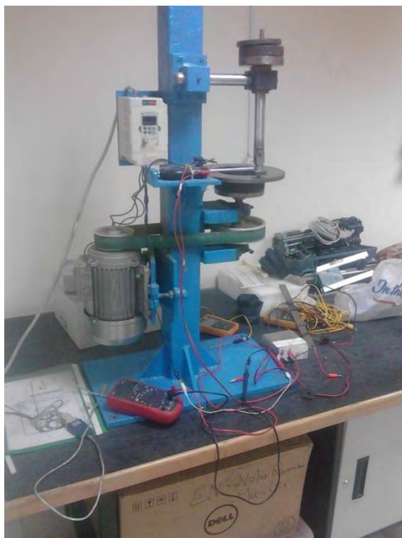
Figure 3.24: Locally Constructed Pin-on-Disc Machine
