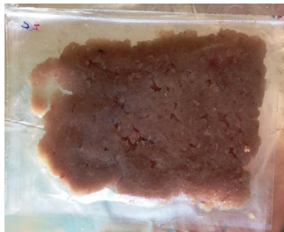
Figure 16. Minced fish sandwiched between 2 layers of PLA
