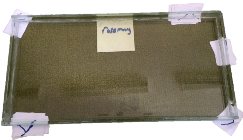
Figure 12. Homogenized solution of PLA, chloroform, tween 80 and rosemary essential oil poured in a leveled glass cast.
