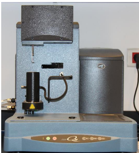
Figure 3.4 TA Instruments, TGA Q50, Center of Materials Science, Zewail City.
