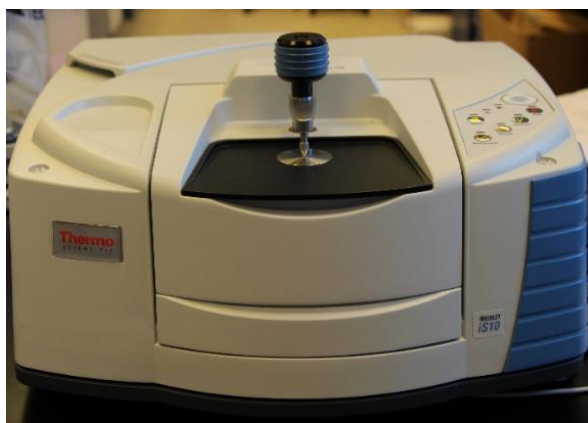
Figure 3.1 Fourier Transform Infrared Spectroscopy, the Center of Materials Science, Zewail City.
