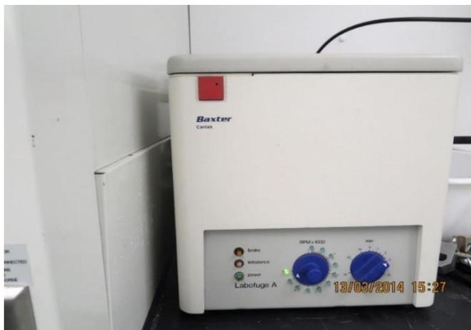
Figure 1.4: A lab centrifuge.
