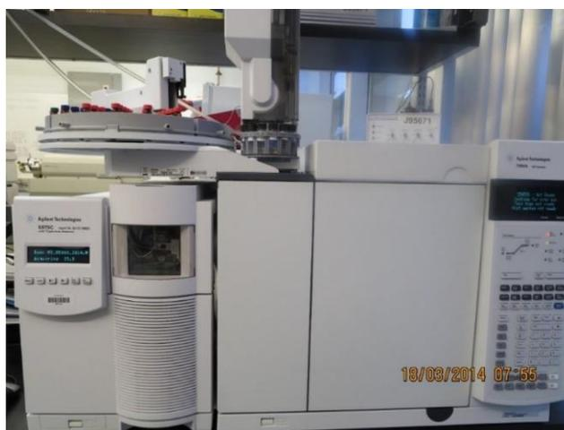
Figure 1.9: Gas Chromatography-Mass Spectrometry apparatus.
