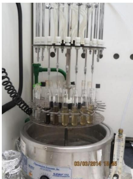
Figure 1.5: Nitrogen blowdown to downsize samples.
