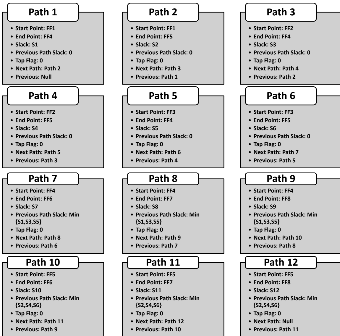
Figure 5.7: The nodes of the bidirectional linked list representing the RTL design of Figure 5.6.
